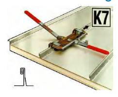
This tool is used for only double standing seam. Ideal for locking short or long runs of roof or wall panels.
