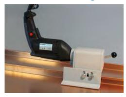
This tool is used for both angle standing seam and double standing seam.
